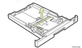
Slide the paper guides to position that match the size of paper you want to load.
