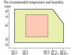
Possible operation range Recommended range To avoid possible build-up of ozone, make sure to locate this machine in a large well ventilated room that has an air turnover more than 30m3/hr/person. If you use this printer in a cold area, leave the printer on. Otherwise, severe cold might damage sensitive components inside the printer.
