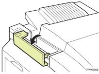
Insert the new oil bottle into the oil bottle case.
