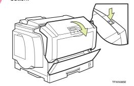
Hold the inset grips (green part) of the photoconductor unit, and pull the top side of the photoconductor unit forward.
