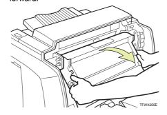
Remove the protective sheet by pulling the red tab from the new photoconductor unit.
