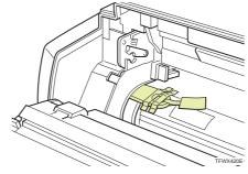
Hold the inset grips (green part) of the photoconductor unit, and push the photoconductor unit to its original position.
