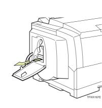
Close the left cover. At this time, the message changes on the panel display. The toner cartridge will automatically rotate to the next color.
