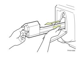
Hold the new toner cartridge and shake it with a horizontal motion, about 10 times, as shown in the illustration.
