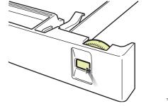
Slide the paper tray completely into the printer.
