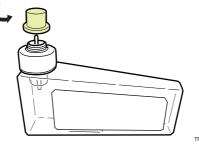
Open the fuser oil bottle cover of the printer.
